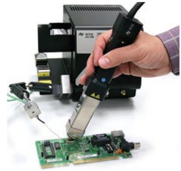
Rapid, simple and safe hand-held component removal
