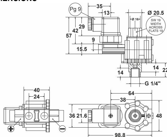
Fig. 2. Dimensions (mm)
