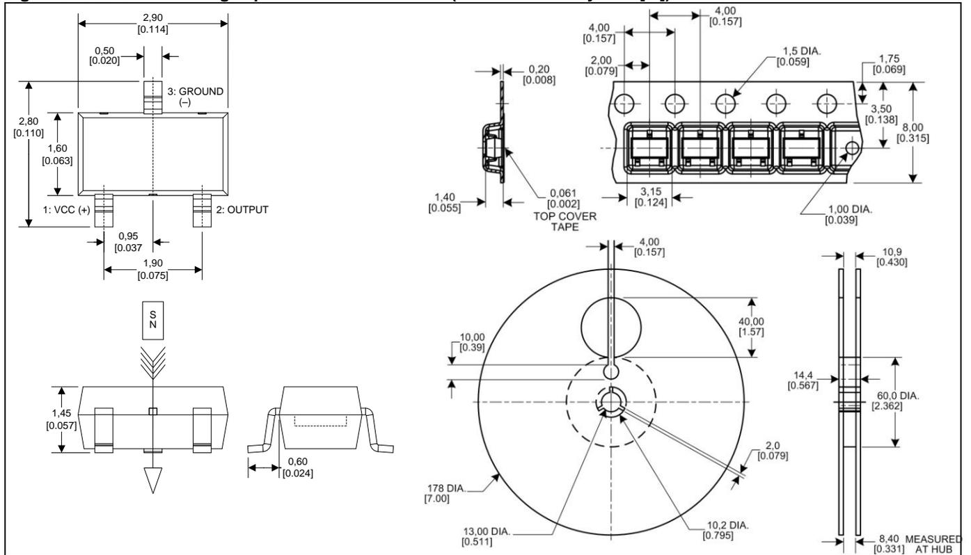
**Figure 4. SS445P Mounting Dimensions (for reference only. mm/[in])**
